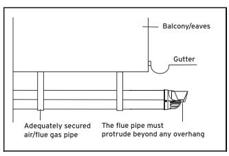
You can use a plume management kit to enable the termination point to be positioned and directed away from the building fabric.
