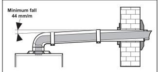
Standard flue terminal kits have an in-built fall back to the boiler to drain the condensate. These can be fitted level between the appliance and the termination position. All other extended flues must have a fall of at least 44 mm/m
