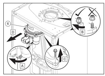
9. Remove the gas-air mixture unit (6).
