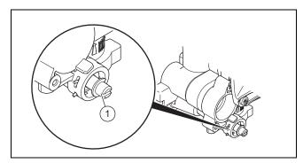
2. Regulate the pressure using the adjusting screw (1).
