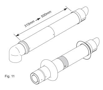
Ensure that no part of the white outer chimney duct is visible
