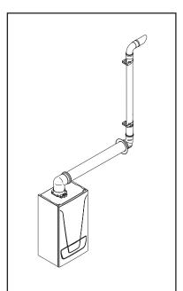
Plume Displacement Kit 60 /100 dia 1M Extensions 45° & 93° elbows are also available - see the separate Flue Guide.
